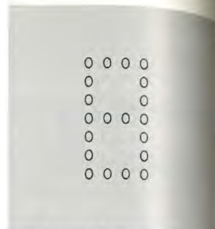
FIGURE 4: Reduced 4 x 7 dot mosaic (20 elements, numeric only).
