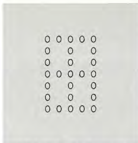
FIGURE 3: Reduced 5 x 7 dot mosaic (27 elements, numeric only).
